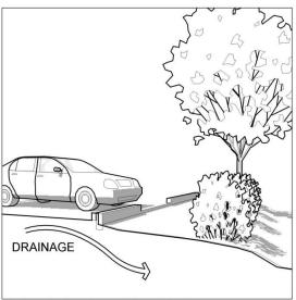
Curb cuts for stormwater drainage
