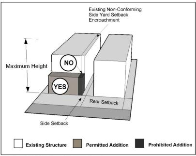
Horizontal Extension of Non-conforming Side Wall
