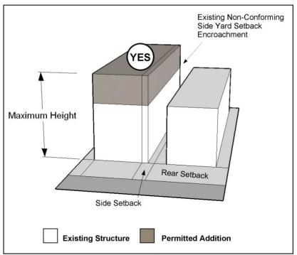
Vertical Extension of Non-conforming Side Wall
