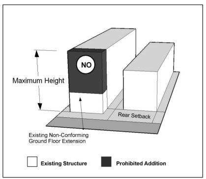
Vertical Extension of Non-conforming Rear Wall
